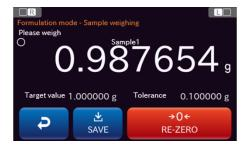
Step 4. Repeat the tare weighing and sample weighing in steps 2 and 3 for every sample registered in the recipe.
