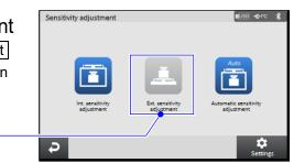
Sensitivity adjustment - Ext. sensitivity adjustment Display settings: MENU key → Sensitivity adjustment button → [Sensitivity adjustment] screen
